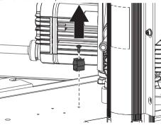
Mount the valve block with earth strap.
