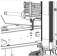
> Remove the clip for L bracket.
